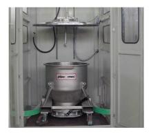
Container washing station using pressurized hot/cold water.
