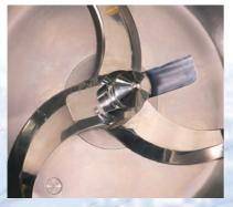
Different rotation speeds for the bottom blade (slow) and the top blade (fast). Speed ratio 1:8.
