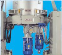
Dual motor with infinite speed ratio.
