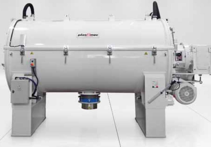
The HEC range of coolers is the ideal solution for all manufacturing needs in the field of rigid or plasticized PVC DRY-BLEND. Available with standard capacities of up to 8.500 liters. The development and optimization of the coolers of mixing plant is the latest PLAS MEC innovation, today it is a straightforward task to cool over 8 batches per hour of U-PVC from 120°C to 40°C.
